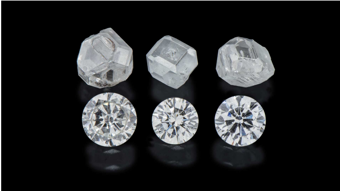
Figure 4: Lab-grown diamond rough (upper row) and polished lab-grown diamond (lower row)
